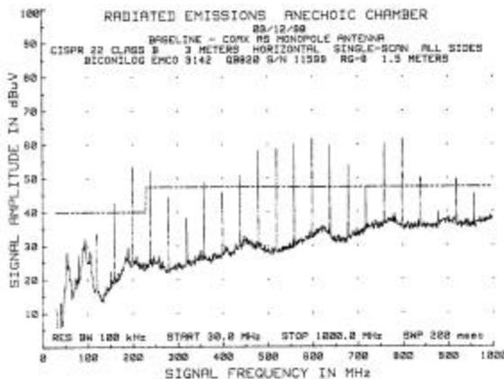
**Figure 5. Baseline measurement of radiated emissions**
