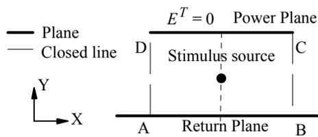
**Figure 4. PCB structure for calculation Poynting vector**
