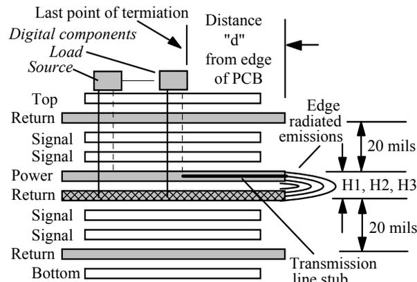
Note: The stimulus source is the last load on a transmission line. Distance "d" to edge of PCB represents an unterminated stub trace in regard to the power and return plane.
