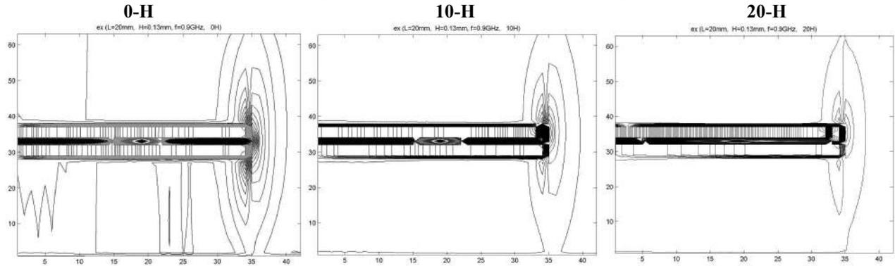
Plots of  $H_y$  with  $L=20$  mm,  $H=0.13$  mm,  $f=900$  MHz (worst case for this configuration – Table 2)
