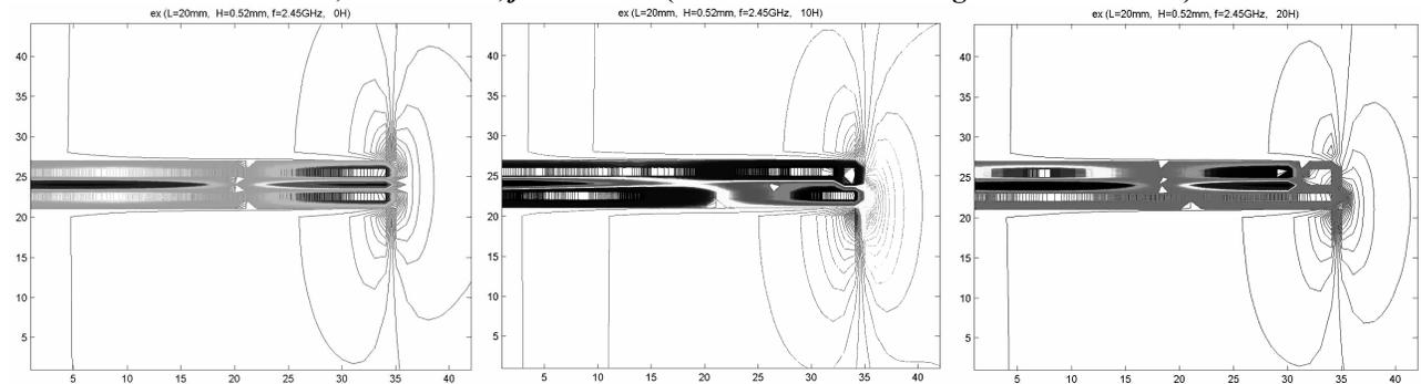
Plots of  $H_y$  with  $L=20$  mm,  $H=0.52$  mm,  $f=2.45$  GHz (best case for this configuration – Table 2)
