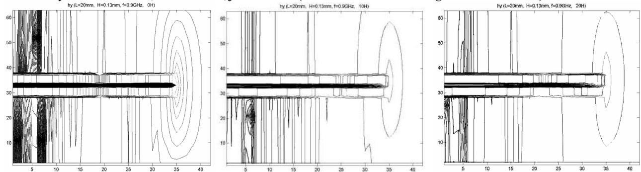
Plots of  $E_x$  with  $L=20$  mm,  $H=0.52$  mm,  $f=2.45$  GHz (best case for this configuration – Table 2)
