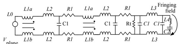
Power and return plane equivalent schematic
