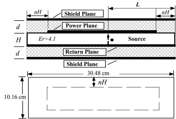
Figure 3. Simulation model
